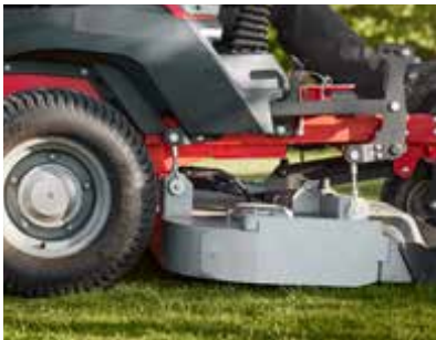
The new rear discharge deck is fabricated from 4.5 mm thick steel with 6.4 mm side wear plates for protection. The blade motor mounting points are reinforced with an extra 3.4 mm layer for additional strength.
