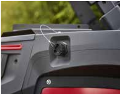
OptimusZ ride-on mowers feature an ETO connection at the front and rear of the machine, allowing for powered attachments such as the ETO Blower or the recharging of batteries.
