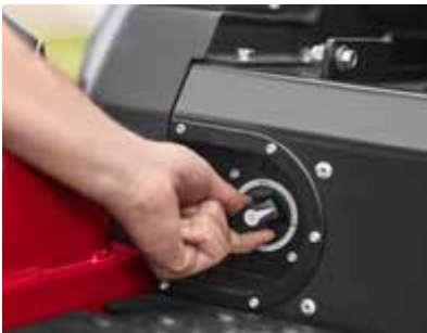
The integrated service switch allows safe access for servicing by isolating the batteries before dealers remove the machine covers.
